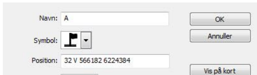
Fig. 23 In the MapSource menu for creating new waypoint you enter the desired name and the coordinate read of (Fig. 22)
